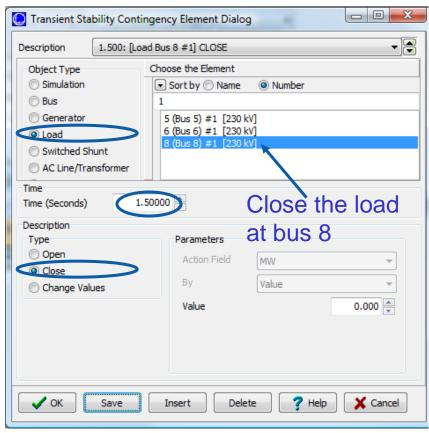
Make events to open the load at bus 8 at 1.0 seconds and close it again at 1.5 seconds
