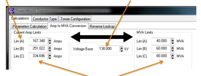
As the user modify either the Amp Limits or the MVA Limits, they are automatically converted
