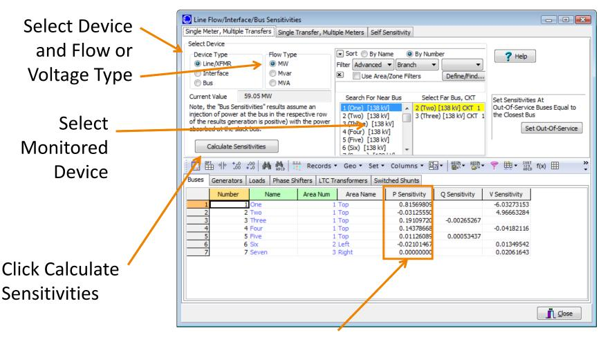
Represents how the Line 1-2's MW will change for a 1 MW injection of Power at respective bus (with the power absorbed at the slack bus)
