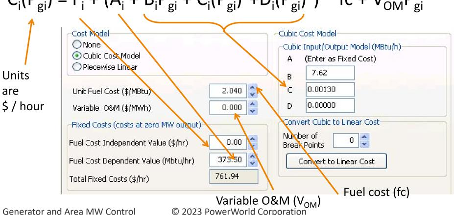
$C_i(P_{gi}) = F_i + (A_i + B_i P_{gi} + C_i(P_{gi})^2 + D_i(P_{gi})^3) * fc + V_{OM}P_{gi}$
