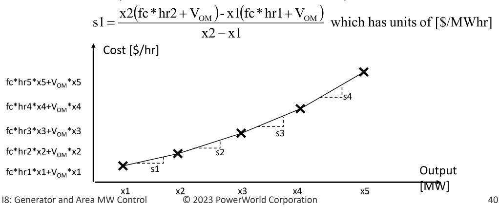
Entering Cost Data in Simulator using a cubic cost model
