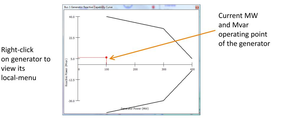
Start the simulation, and then use the spin button to the right of the generator to change the MW output of the generator. Notice how the operating point on the graph changes.
