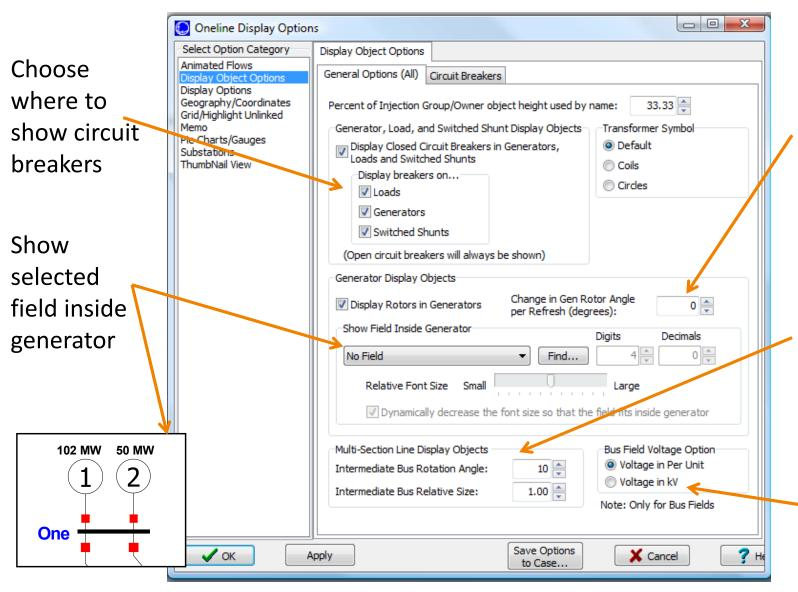
Each time the display refreshes, the generators "rotor" will rotate this amount
