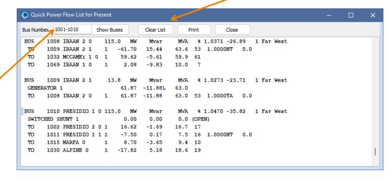
Circuit identifier 99 indicates an equivalent line
