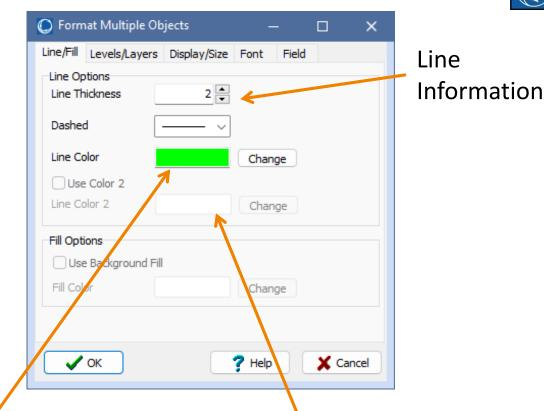
Color 2, used with transformers (i.e. for different voltage levels)
