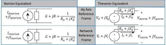
Conversions between reference frames are done using equation 6.8 and 6.9 on page 125 of Sauer/Pai book. The same general function works for converting all phasors between the dq axis and network reference frames. Assume you have a complex phase F that can be written as either  $F_d + jF_q$  or  $(F_r + jF_i)$ .
