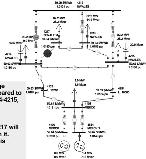
4217-4216 line has a large impedance of 0.15 compared to the lines 4214-4217, 4214-4215, 4216-4215 which have impedances of 0.0002
