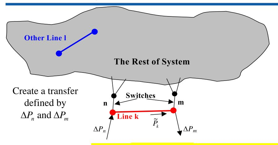
Assume  $\tilde{P}_k = \Delta P_n = \Delta P_m$ Then the flow on the Switches is ZERO, thus Opening Line K is equivalent to the "transfer"
