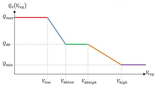
Within PowerWorld Simulator, we constrain this function with a voltage tolerance (Tol) and also the relationship of reactive values using the following code which ensures that the curve is a nonincreasing function of voltage, and also that it is not too steep a derivative!
