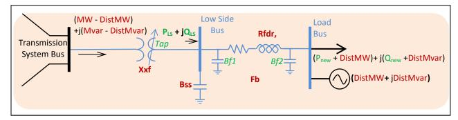
The initialization of the distribution equivalent is performed the same way as described earlier but net load at the transmission bus is Load – DistGen instead. The value of  $P_{\text{new}}$  and  $Q_{\text{new}}$  is done the same, however during the processing when the loads characteristic models are initialized, the MW and Mvar at the Load bus is split between the load characteristic and the load distributed generation model as follows.
